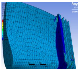
Figure 11: Directional Heat Flux distribution over the Turbine Blade Profile.
